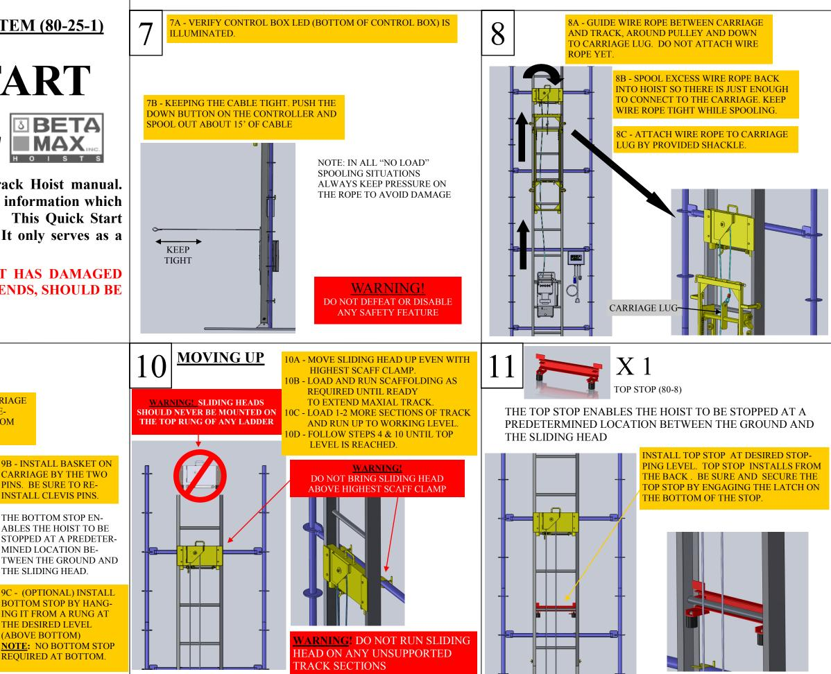
X 1 BOTTOM STOP (80-4) 9A-LOWER CARRIAGE BY FIRST RAISING THE CARRIAGE TO RELEASE THE BRAKE. NOTE WEIGHT MAY BE RE-**OUIRED ON THE CARRIAGE TO KEEP THE BRAKE FROM** ENGAGING IN THE DOWN DIRECTION. **9B - INSTALL BASKET ON** CARRIAGE BY THE TWO PINS. BE SURE TO RE-INSTALL CLEVIS PINS. THE BOTTOM STOP EN-ABLES THE HOIST TO BE STOPPED AT A PREDETER-MINED LOCATION BE-TWEEN THE GROUND AND THE SLIDING HEAD. 9C - (OPTIONAL) INSTALL BOTTOM STOP BY HANG-ING IT FROM A RUNG AT THE DESIRED LEVEL
