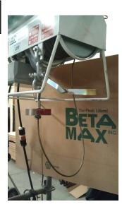
Connect the Jaw/Eye swivel to the double rope tab on the hoist. Then connect the wire rope to the Jaw/Eye swivel with the original shackle. Be sure to bend over the cotter pin on the Jaw/Eye swivel and make sure all pins are tight
