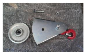
2.1) Unbolt the pulley keeping track of all components so they may be re-assembled in the same position as they were dis-assembled (eg. Bolt, nut, pulley, bearing(s), spacer(s), and washer(s)).
